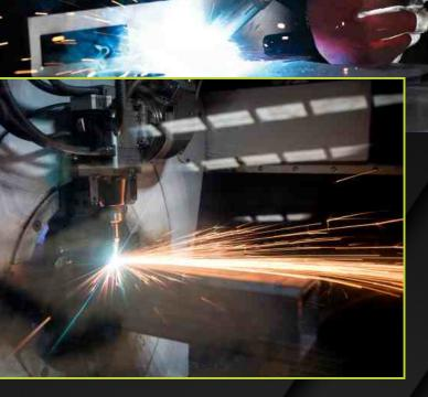
We start with steel tubing which is cut using lasers for 100% accuracy. Then, the parts are welded into a massive steel frame which is powder coated for a superior protected finish.
